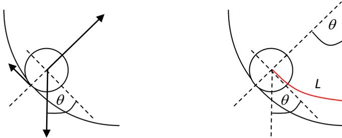
Friction provides the torque:
